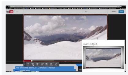
Screencast allows content from any desktop, including web pages, to be displayed on-air in real-time. Viz Engine, Vizrt's real-time compositing engine takes Screencast content and distributes it as an HD SDI output. The combination of Viz Engine, Screencast, and a scan converter is all that is needed.
