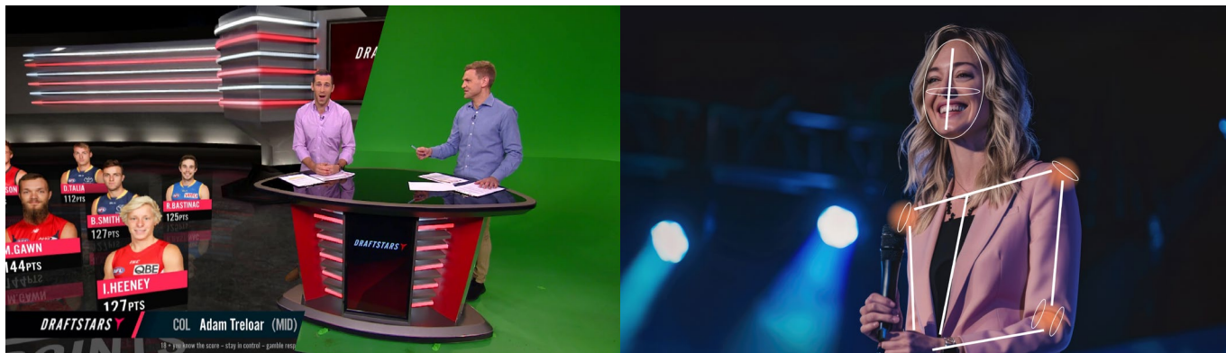
AI-based real-time pose estimation enables realistic talent reflections and shadow casting, produced by Reality Connect™, natively in Viz Engine 5.
